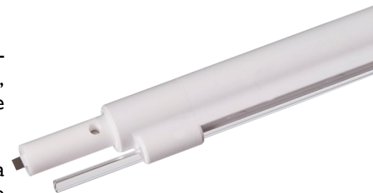
Tip of sampling wand, showing blade and capillary tube
